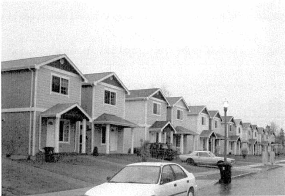
Figure 15-1. Avoid monotonous configurations like this where identical setbacks are used along grid streets.
