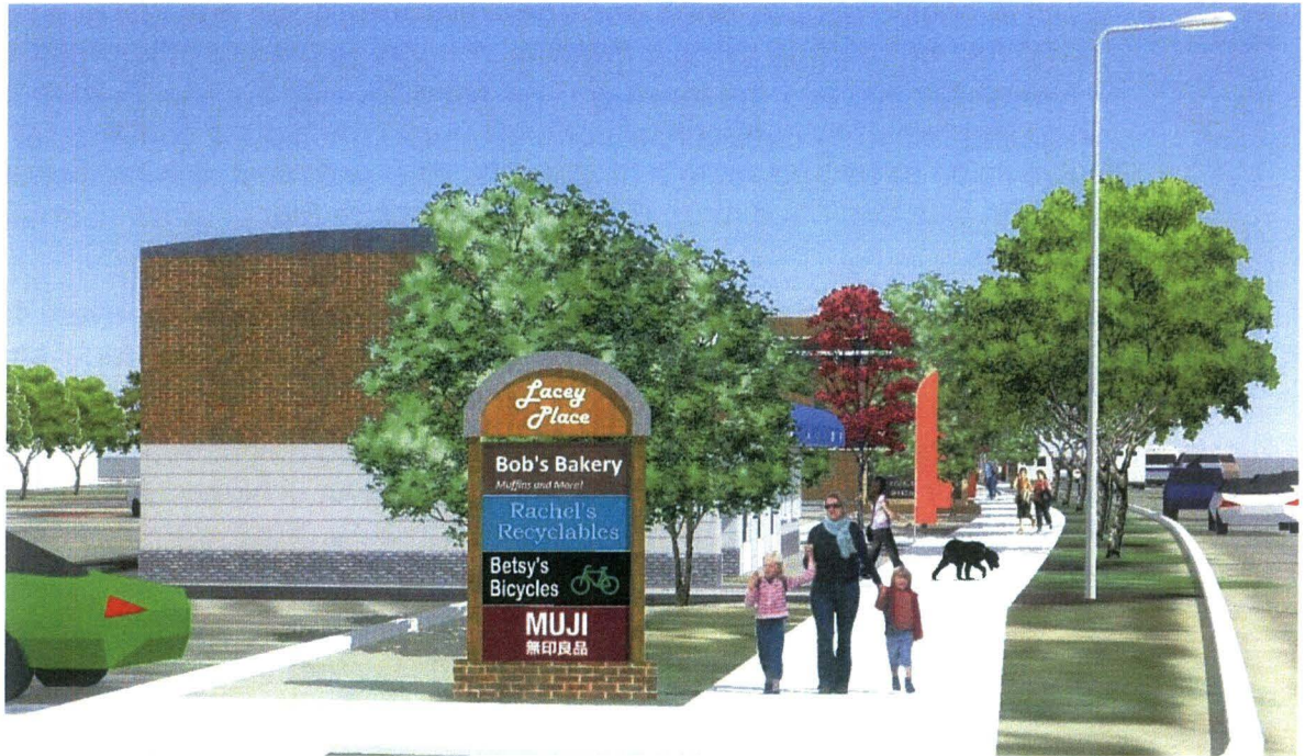
Figure 16.75.080(A)(8)(b-2). An example of a 24 square foot sign in a 35 miles per hour zone meeting the maximum 12 pieces of information requirement. Note that the center name “Lacey Place” does not count as an item of information.
