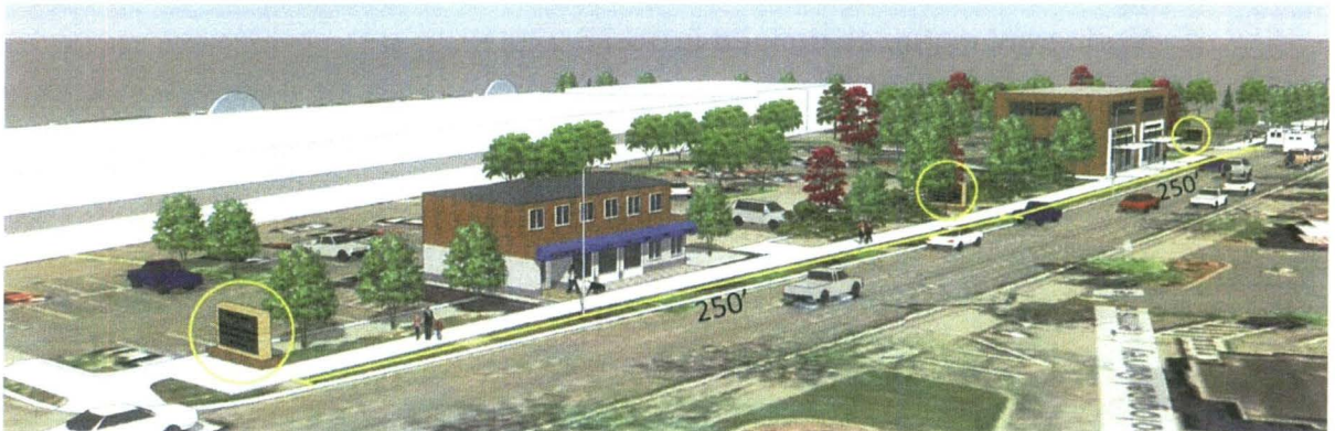
Figure 16.75.080(A)(3). An example of a shopping center with a large frontage where multiple freestanding signs are allowed. The fronting street has a posted speed limit of 35 miles per hour, which requires a minimum sign separation of 200 feet.
