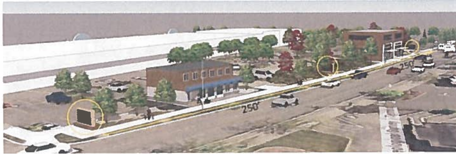
Figure 16.75.080(A)(3). An example of a shopping center with a large frontage where multiple freestanding signs are allowed. The fronting street has a posted speed limit of thirty-five miles per hour, which requires a minimum sign separation of two hundred feet.
