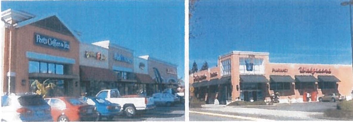
Figure 16.75.080(B)(3-2). More acceptable wall sign examples. In the right image, the signs are centered on the articulation elements of the facade.
